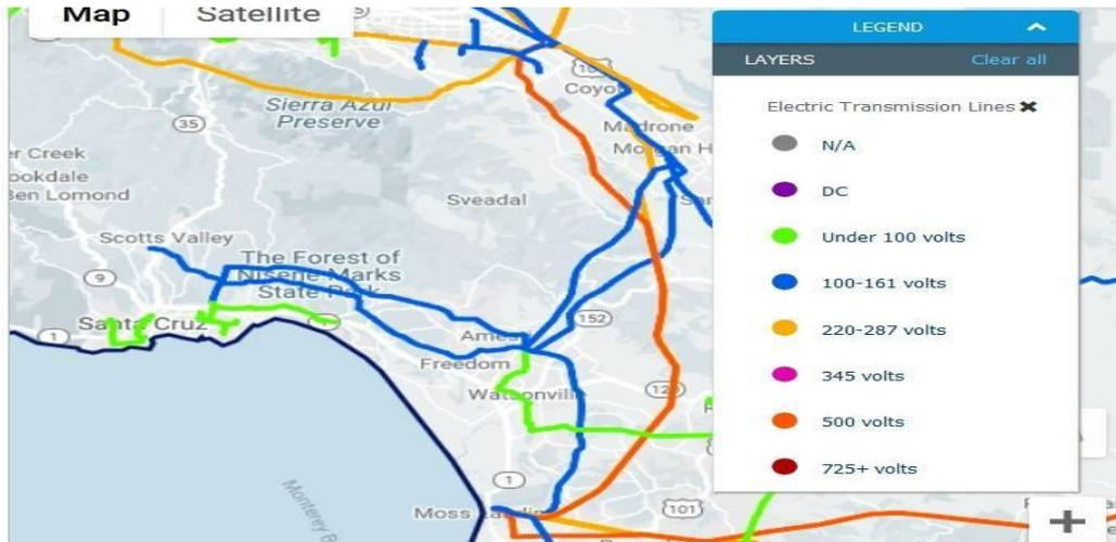
Figure 2: High-voltage power lines feeding the Santa Cruz Area<sup>4</sup>
